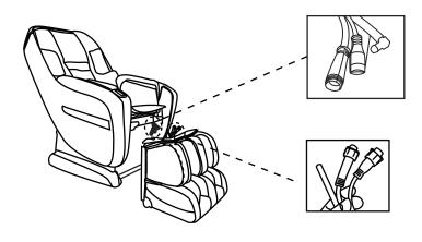
Step 2: Align the connecting holes from the footrest and seat part, insert a flat head rivet and secure with a split pin as demonstrated.
