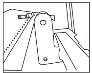
Step 3: Attach the connecting rods of the seat part and footrest with a flat head rivet and secure with a split pin as demonstrated.
